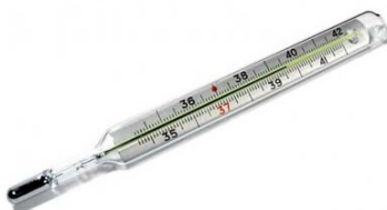
Mercury Fever Thermometer; Photo Source: Utah Department of Environmental Quality (UT DEQ)
