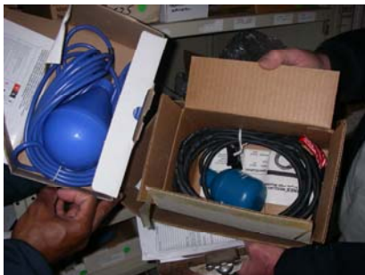
Float Switches for Sump Pump System; Photo Source: NEORS D
