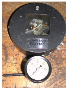
Pressure Gauge Photo: Cuoco & Cormier
